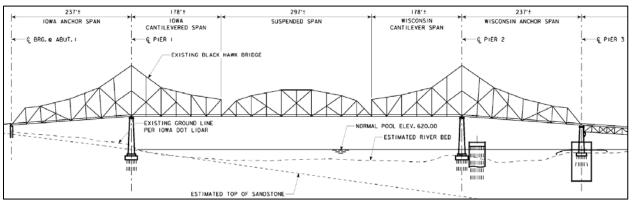
Figure 4. Diagram of south elevation of the Black Hawk Bridge main structure. Note the estimated depths of river bed and bedrock relative to the depths of the piers. This diagram shows the anchor and cantilever arms as separate spans. Source: Burns McDonnell 2019:8.
