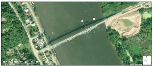
Figure 2. Current aerial showing main spans of bridge and approach spans leading to causeway. Two dolphins can be seen north of two piers on Wisconsin side of channel. Source: ExpertGPS mapping software, accessed August 2022.
