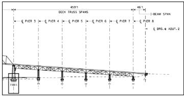
Figure 15. Diagram of south elevation of the east approach spans and east part of main structure. Source: Burns McDonnell 2019:8.
