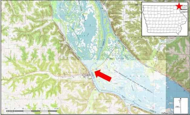
Figure 3. USGS topographic map showing the Mississippi River (main channel marked by line of Iowa-Wisconsin border) and the Black Hawk Bridge (red arrow). Note the many sloughs to the east part of the bridge structure, and the near-90-degree turn in the main channel to its north. Inset: Map of Iowa counties showing project location (red star) in Allamakee County. Source: ExpertGPS mapping software, accessed August 2022.
